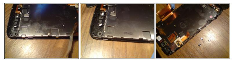
Loosen any clamps that hold the LCD screen in place. Some of the clamps may not be loosened yet, leave them attached for now.
