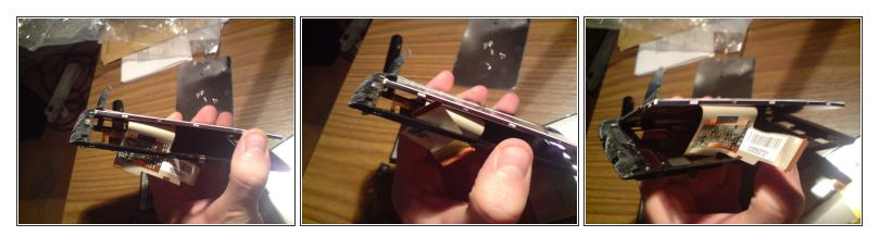
• Lift the new display out of the case. You should fold the LCD ribbon cable to do this.
