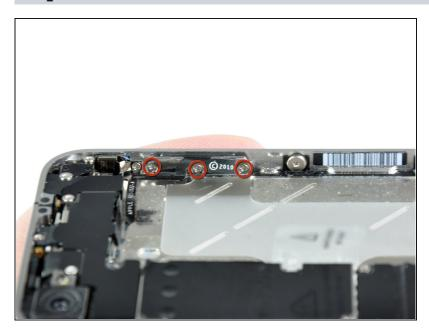
Remove the three Phillips screws securing the volume button bracket to the outer case.
