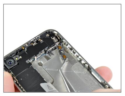
Use a pair of tweezers to gently pull the volume button bracket slightly away from the outer case.
