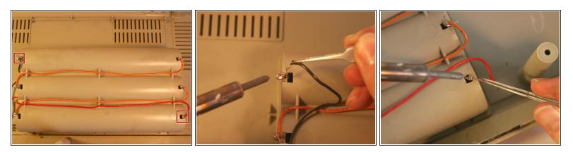
Unsolder the wires connecting the power supply unit to the battery container.
