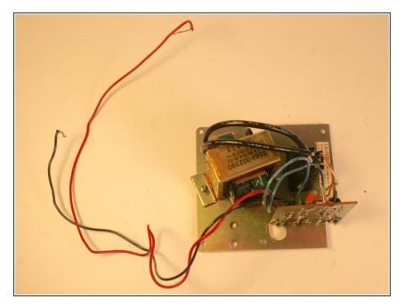
• Remove the power supply unit.
