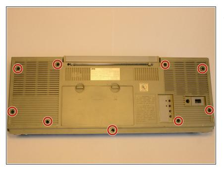
Remove the nine 35 mm Phillips screws securing the back cover of the case.
