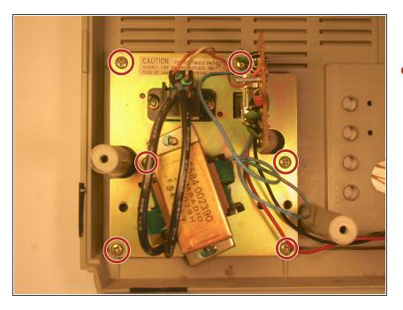
Unscrew the six 10 mm Phillips screws holding the mounting plate in place.
