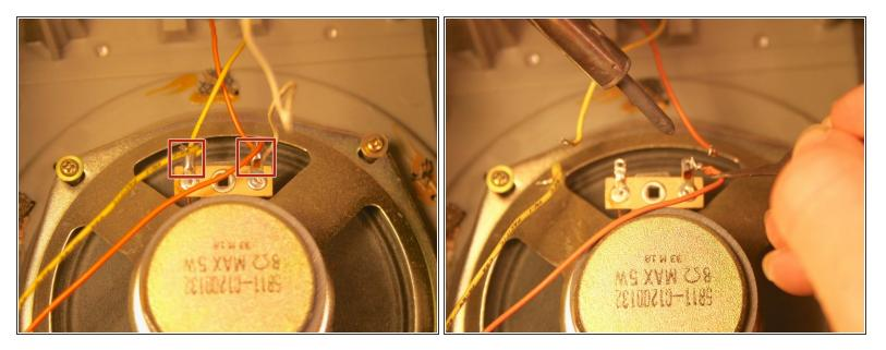
Unsolder the wires leading to and from the subwoofer.
