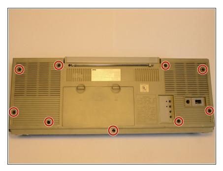
Remove the nine 35 mm Phillips screws securing the back cover of the case.
