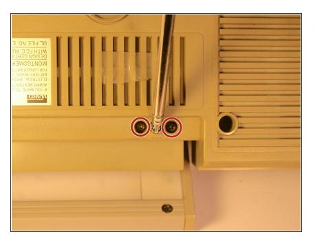
Tilt the back cover up and remove the two 7.5 mm Phillips screws holding the antenna in place.
