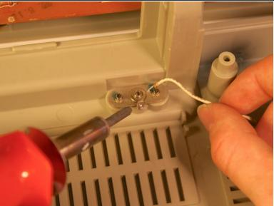
Unsolder the wire connecting the antenna to the radio.
