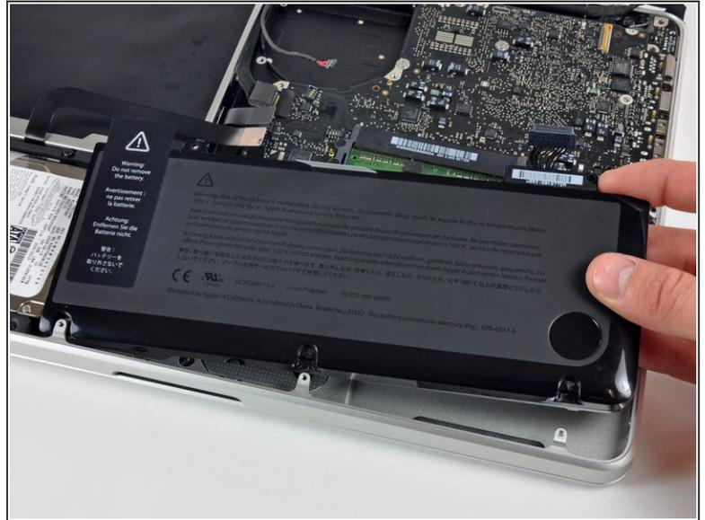
**i** Removing the battery before lifting out the logic board is not strictly required, but makes removing the logic board easier and safer. If you leave your battery in, be especially careful not to bend the logic board against the battery's case near its bar code.
