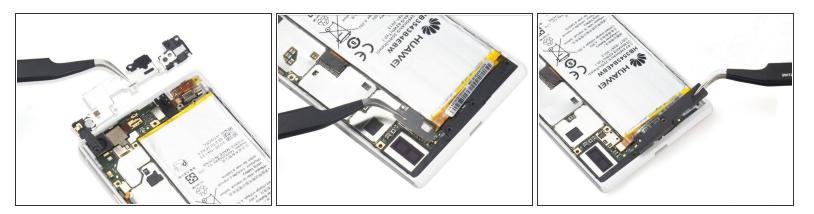
• Remove top bracket, battery bracket and USB bracket cover.
