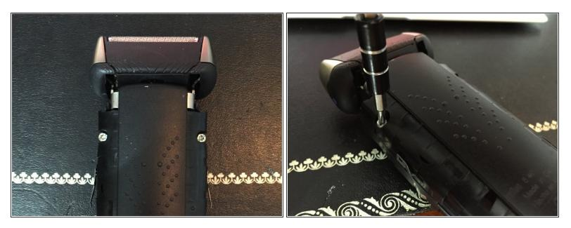
Remove the 4 screws that are now exposed on the back of the shaver. You will need a T9 hex screw driver.
