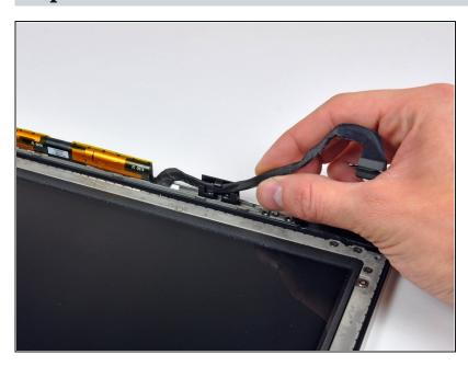
De-route the display data cable from its retaining bracket near the lower left edge of the display.
