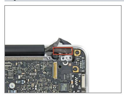
(i) If present, remove the small strip of foam tape stuck to the display screws near the display data cable.
