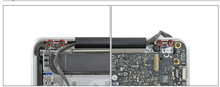
• Remove the two outer 6.5 mm T8 Torx screws securing each of the two display brackets to the upper case (4 screws total).
