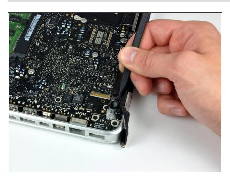
Use the tip of a spudger to pry the microphone off the adhesive attaching it to the upper case.
