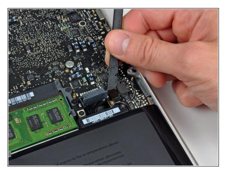
Use the flat end of a spudger to pry the battery indicator cable connector up off the logic board.
