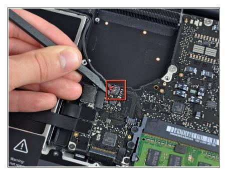
Use the flat end of a spudger to pry the subwoofer and right speaker connector up off the logic board.
