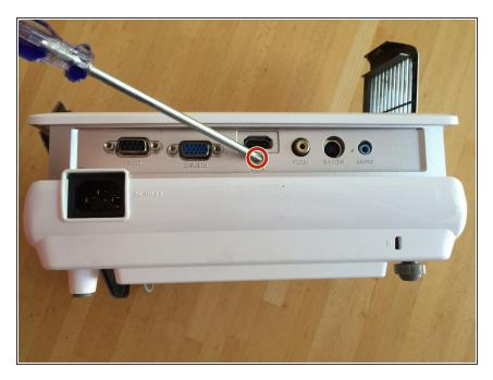
Remove the Phillips screw on the back of the projector.
