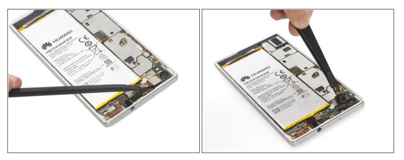
• Release the connector and remove front camera.
