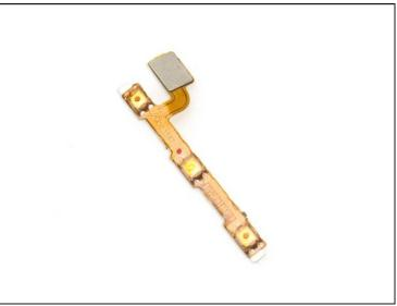
• Use the <u>tweezers</u> or some tools thin and sharp to cut the adhesive between power flex and bracket. And then pry it up and remove it.
