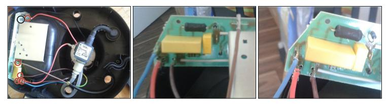
• Disconnect all cords from the circuit board besides the two black ones on the right(marked black on the first picture); these are soldered and therefore cannot be disconnected so easily.
