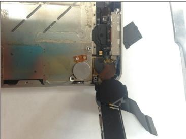
Use the spudger again for the battery connector that covers the logic board to disconnect.
