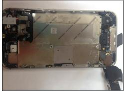
• Use the ifixit opening tool to remove the screws that hold the logic board in place and lift it with sprudgers in order to completely remove it from the Iphone (This will require some force when lifting the logic board).
