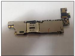
• There will be the EMI Shields on the logic board (metal on top of the main processing chips) Which a spudger or the opening tool could be used for removal by lifting the small multiple metal tabs on the sides.(This will require *a lot* of force to lift off the logic board) (May cause a cut if not done without caution)
