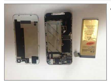
Pyou'll automatically see the battery when taking of the back glass(will show a recycle sign and Li-ion written across). There is a plastic tab for you to use to help carefully lift the battery out of the phone (The battery has a connected wire to it, but it can be easily disassembled).
