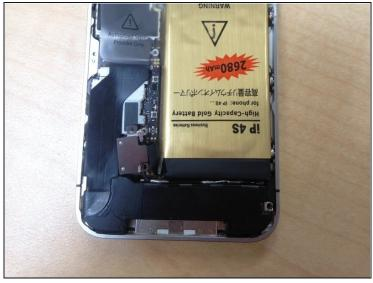
• The iPhone will open up and you will see a metal panel by the camera on the top left side of the phone as well as a smaller metal panel on the bottom left side of the phone. These are required to be removed before taking out the battery. A Phillips #000 screwdriver will work best for removing them.
