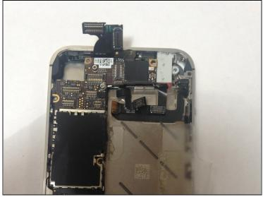
• This is where you'll need your spudger, this will help you lift and disconnect your camera as well as other connectors which you can remove with <u>tweezers</u> (delicate part). With your spudger, you will go <u>under</u> the connector in order to lift and remove the camera from the logic board.
