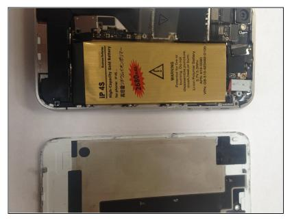
Make sure to <u>push up</u> on the back glass when taking it off (<u>be careful</u> if the back glass is cracked, loose glass could come off and potentially cut your hand if not done right)
