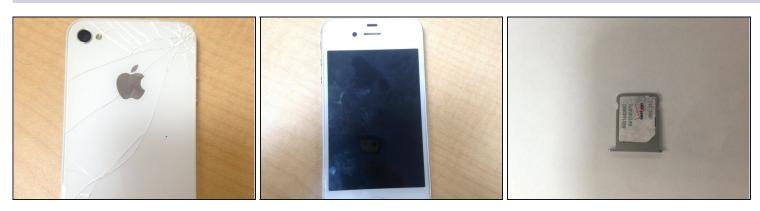
• Use a 5-point Pentalobe Screw (only for iPhones)to remove the bottom screws on the iPhone 4S. For the Sim Card Holder, there will be a small hole which you can use a remover tool, (or paper clip, which is not the safest tool to use), but will require a fair amount of force for pushing into the hole get the holder out.
