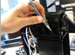
Disengage the tabs holding the top assembly to the case.
