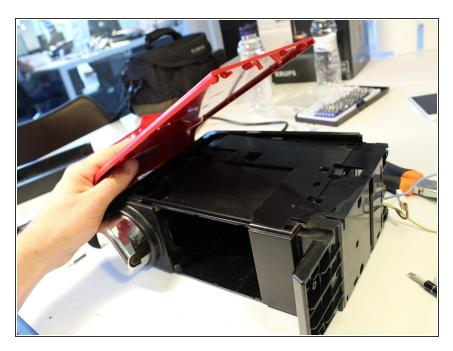
Remove the side panel from the other side of the unit. The tab positions are similar to the first side panel.
