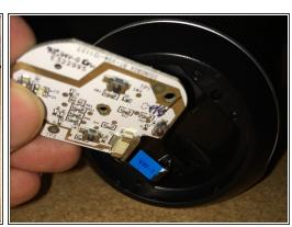
Replacement of original 7.4V batteries of 1000mhA each for two Blackberry 8520 batteries of 2450mhA
