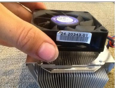
Remove the four screws from the heatsink fan and remove the fan.
