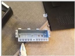
Remove the two screws on the audio box. Then pull it out and set the case aside.
