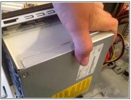
Remove the four screws from the power supply and then pull it back and out
