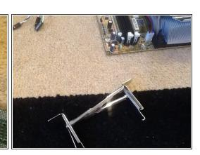
Remove the Heatsink clips by pushing down and out on the clips.
