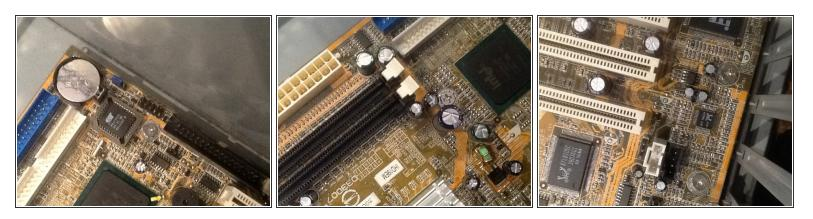
Remove the six screws from the motherboard, one in each corner and two in the middle in between these
