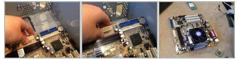
Grasp the motherboard by the side that would face the front of the computer, and pull it towards the front, and then up.
