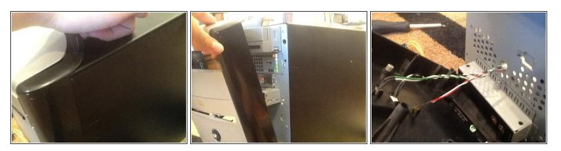
To remove the front panel, Grasp the top, and pull it outward and upward.
