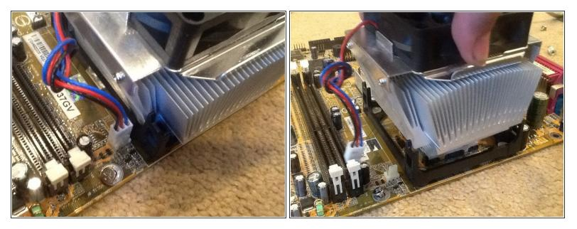
Disconnect the fan cable and lift the heat sink up
