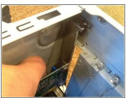
Remove the single screw securing the phone card. Then pull it up and out.
