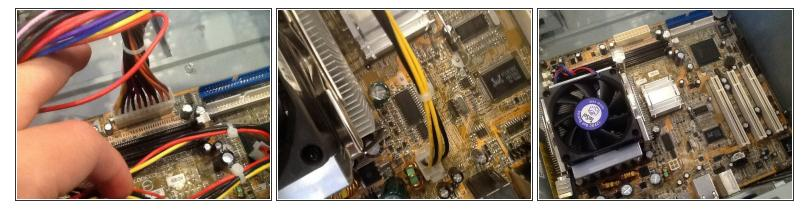
Disconnect the 20 Pin motherboard cable and the four pin cable.
