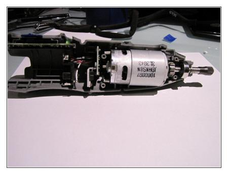
You can remove the buttons except for the sliding one that adjusts the speed
