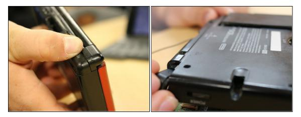
• Also remember that following this, you need to remove the left and right trigger buttons from their sockets.
