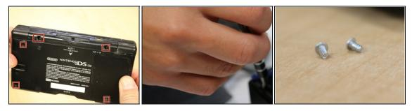
• Using the Phillips head screwdriver, remove any and all screws from the back ports of the DS.
