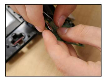
Now take the black and white wires present near the Wi-Fi Board, and start with placing your spudger thumbnail on the black wire.
