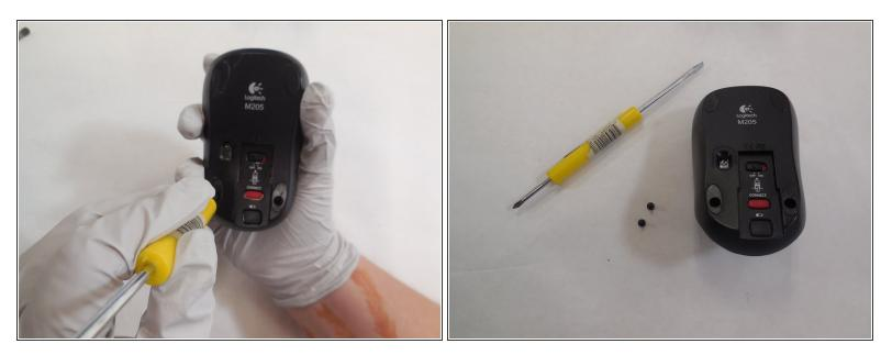
Using a phillips head screwdriver (J000 in ifixit toolkit), unscrew the screws holding the base in place.
