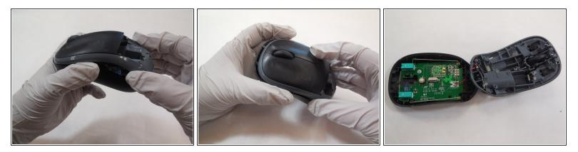
Lift up the back side of the mouse, then gently slide the front towards the back.
