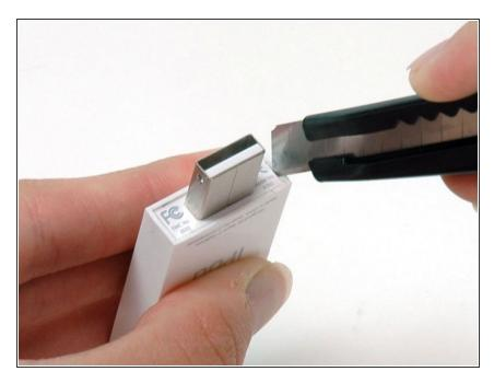
Continue to run the knife around all four edges of the USB port until the glue is released. You may be able to gently wiggle the knife from side to side to help release the glue.
