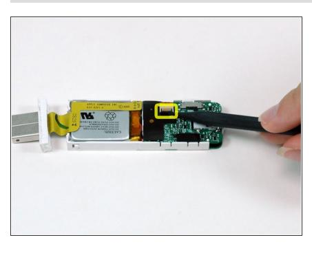
Use a spudger to flip up the black plastic tab holding the USB port ribbon in place. The black tab will
