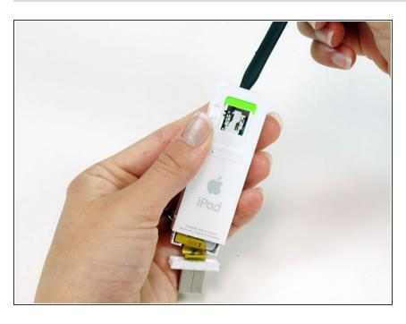
Continue to slide the iPod out of its casing by using a spudger to push on the logic board near the headphone jack.
