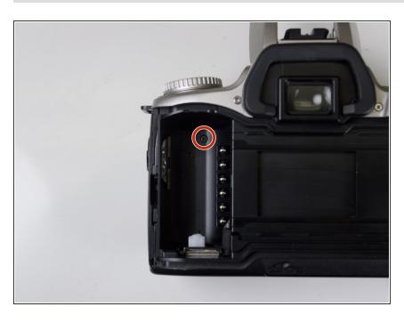
Remove the black Phillips #00 5.0 mm screw from the back of the film compartment.
