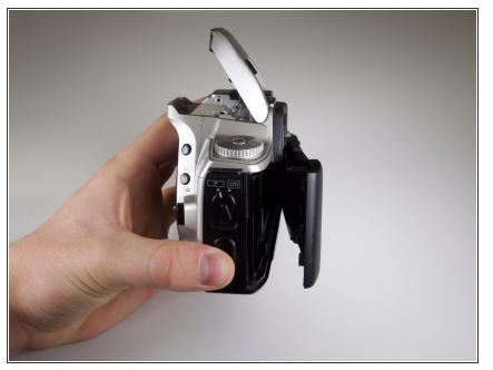
Press up firmly on the back-cover release on the right side of the camera to release the back panel.
