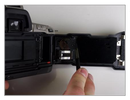
• Use tweezers to lift off the battery compartment cover.
