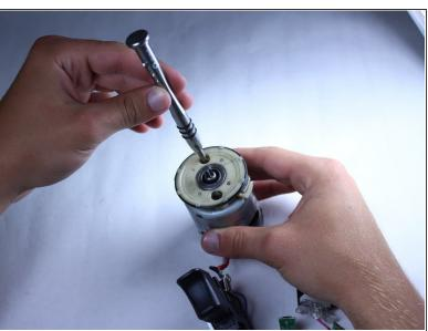
Remove the two 14 mm long PH1 screws that connect the plastic object to the motor assembly.
