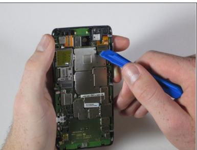
Disconnect the snap connection in the upper right corner by prying underneath using the plastic opening tool.
