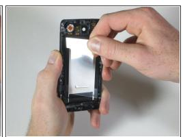
Peel back the plastic from the face of the battery.
