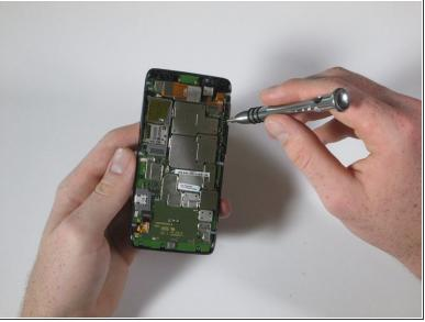
Remove the six 4mm T5 Torx screws located along the outer edge of the motherboard.
