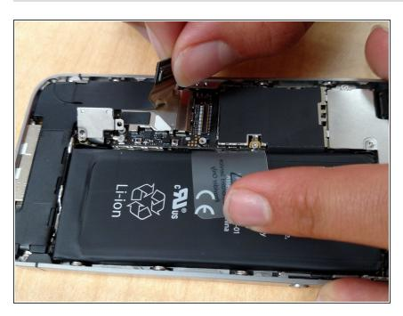
Use the head of your tool to remove the dock cable up from its socket on the logic board.
