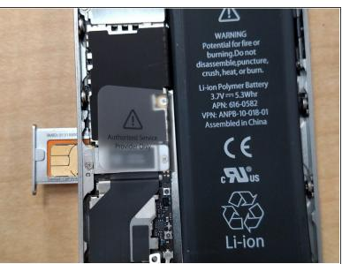
Use a paper clip to eject the sim card and put it in a safe place
