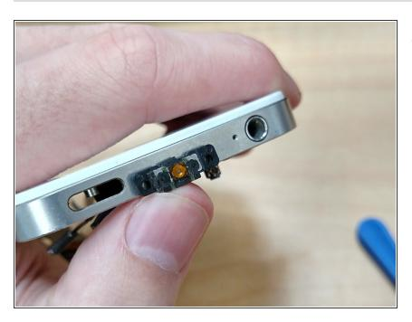
Once done, remove the power button with either tweezers or a sharp object
