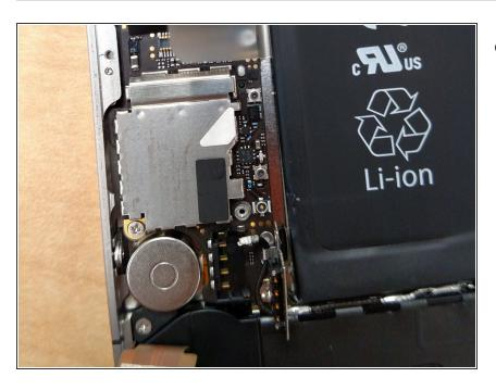
Once pulled up, Peel the dock connector cable off the logic board
