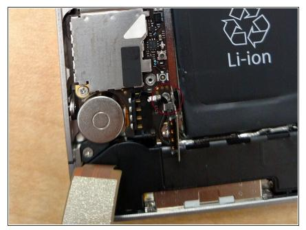
Unplug the cellular antenna cable out from under the metal fingers attached to the logic board and place it on the same side as the doc connector cable
