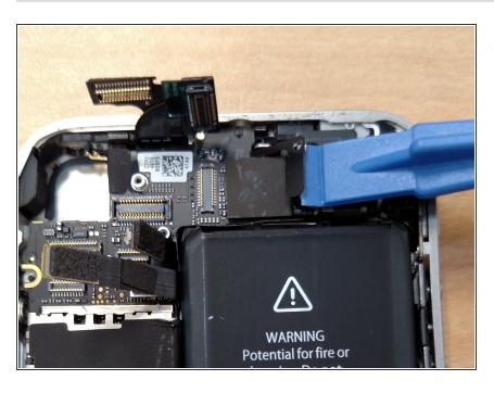
Pry up the small grounding clip with the head of your tool and then remove it and put it in a safe place
