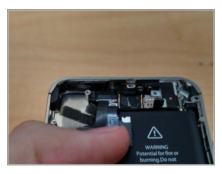
Take out the two screws keeping the lock button in place
