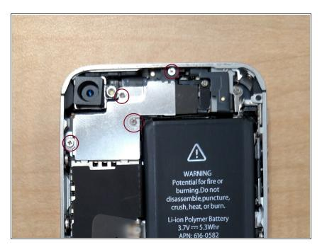
Take out four screws securing the cable cover to the logic board (the screws highlighted)
