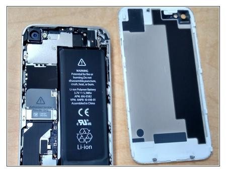
Carefully pull the rear panel away from the iPhone. Be careful not to break the clips that attach it to the phone.
