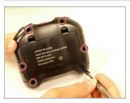
Remove the six Phillips #0 screws from the back of the remote.
