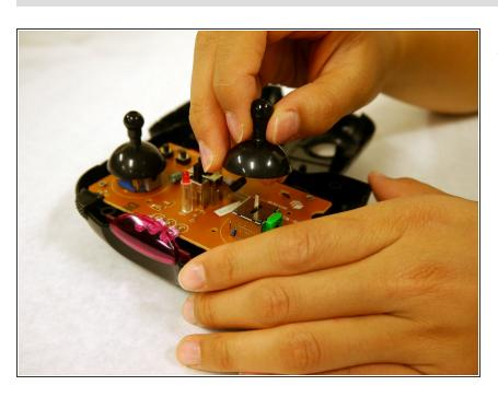
While holding the remote down with one hand, pull the joystick up with the other hand to remove it.
