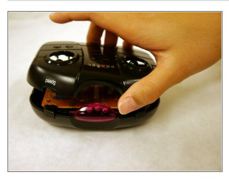
With the joysticks facing up, lift up the top of the remote casing to remove it.
