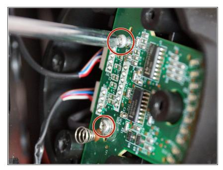
Remove the two 7.5 mm silver screws holding the green PCB board in the wheel with a Phillips #1 screwdriver.
