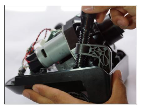
Unscrew the piece holding the C-Clamp in place with your hand.
