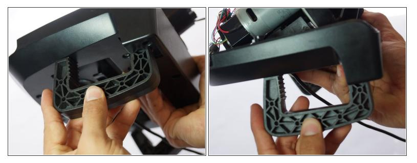
• The C-Clamp can now be easily pulled out of the bottom of the device.
