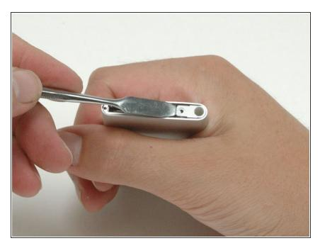
Use a metal spudger to carefully pry the headphone jack out of the casing. DO NOT remove the headphone jack from the iPod entirely, as it is connected via a fragile ribbon connector to the click wheel.
