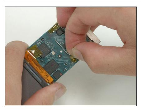
Peel up the orange tape covering the three solder points on the other side of the logic board.
