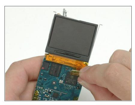
Peel up the orange tape covering the display ribbon cable.
