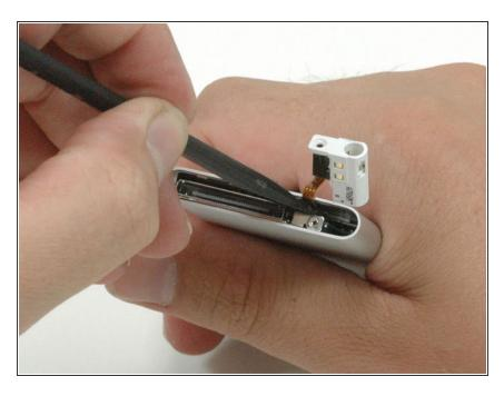
Use a spudger to disconnect the headphone jack cable from the logic board. You need to gently pry the connector toward (or up, if you like, the connector is like LEGO® building blocks) the front of the iPod until it comes loose from the logic board.
