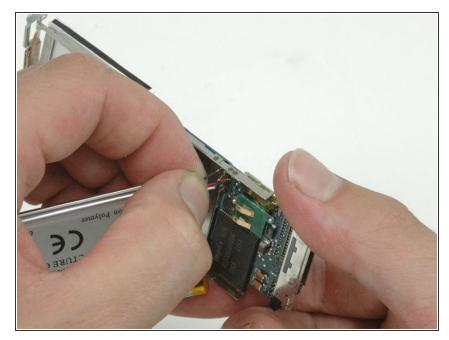
Pull the battery wires through the logic board to free the battery. If the wires don't easily come free, make sure the wires are straight and all the solder has been removed.
