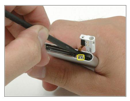
When removing the logic board, place the tip of the spudger into the hole where you removed the screw and gently push it out. The crevice will keep it in place and decrease the chance of you damaging your board.
