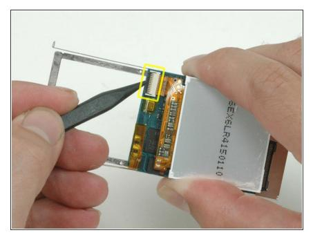
Use a spudger to flip up the black plastic tab holding the orange display ribbon in place. The tab will rotate up 90 degrees, releasing the ribbon cable.
