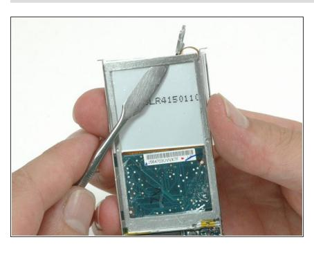
Use a metal spudger to carefully pry the metal bracket off the back of the display. Make sure you only pry off the bracket and not the clear shielding on the rear of the display. By working from the inside of the display, you won't be able to accidentally pry up the clear plastic shielding.
