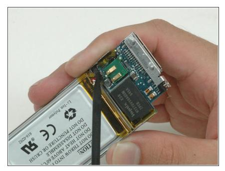
Use a spudger to scrape away the black glue covering the three battery wires.
