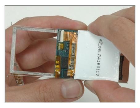
Slide the display ribbon out of its connector and lift the display off of the logic board.
