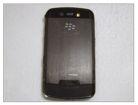
Turn your Blackberry Storm 9500 onto its back side, and remove the battery door & battery.
