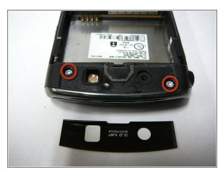
Once the plastic piece is removed, unscrew the two torx screws underneath it.
