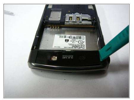
Flip it back over to the back of the phone, and remove the plastic lens on top of the camera & flash. This is held in place by some adhesive, so use a safe pry tool to remove as shown.
