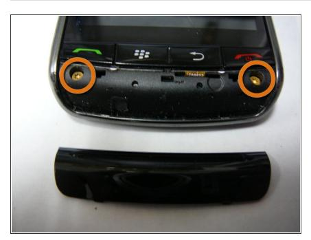
Remove the two screws(T6) as shown.
