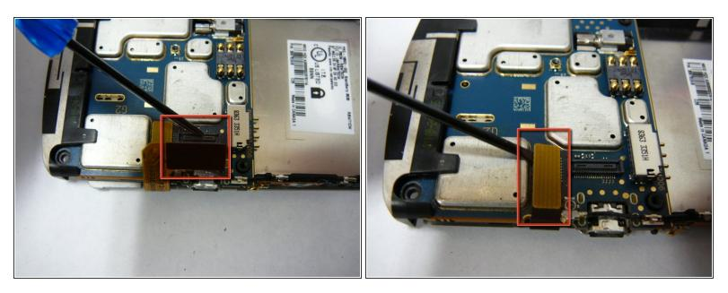
• Flip the logicboard around so that it is sitting on top of the screen, now remove the two ribbon cables for the LCD & Digitizer.
