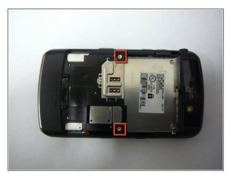
Remove the 2 screws (T6) under the battery compartment they are located as shown in red.
