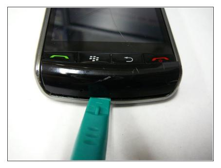
Turn the Blackberry Storm 9500 around and pry off the microphone cover at the top using a safe pry tool.
