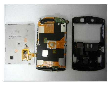
Now remove the logic board & LCD assembly from the rear housing. Be gentle, and do not use excessive force.
