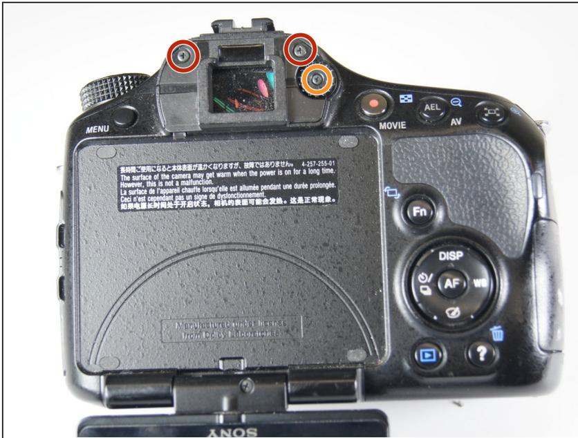
**!** Be careful when pulling the back panel away as it will still be connected to the body of the camera by two strips of film.
