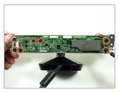
Unscrew the seven 6.5mm T10 Torx screws.
