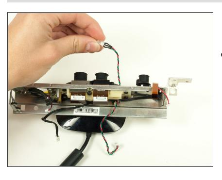
Gently pull the LED out of the front of the metal casing. It should slide out easily. To reassemble your device, follow these instructions in reverse order.
