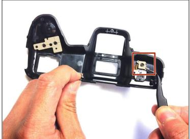
Gently remove the beige rubber tabs from under the casing by pulling each down using tweezers.
