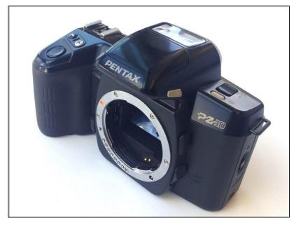
i The top cover is one piece encasing the top of the device except the shutter release button and flash.
