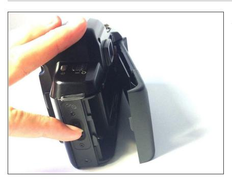
With the door unlocked, rotate the device to access the bottom.
