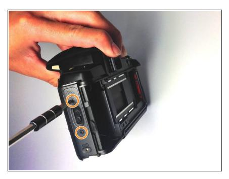
Once the back cover is fully removed, remove the two 4.35mm screws attaching the cover of the unlocking switch, and remove the plate.
