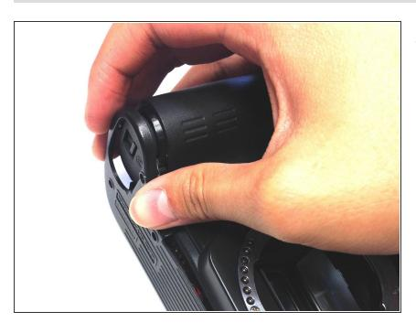
With the screws removed, the bottom casing should come off very easily by pulling on the casing.
