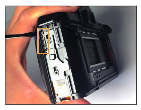
Locate the spring at the upper left corner of the face, and pull the rings of the spring off of the pins to
