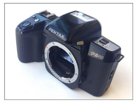
The top cover is one piece encasing the top of the device except the shutter release button and flash.
