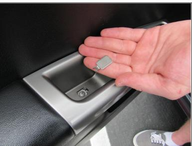
Pry up the plastic tab from inside the handle located on the front door armrest.
