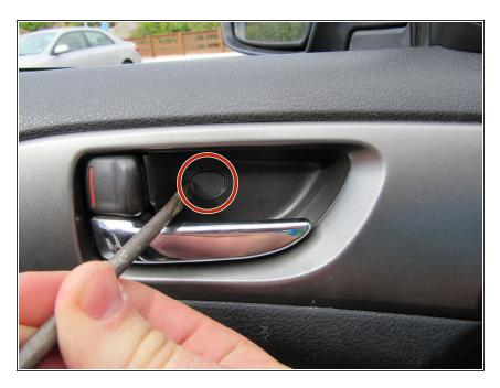
Pry up the plastic tab from inside the door handle housing.
