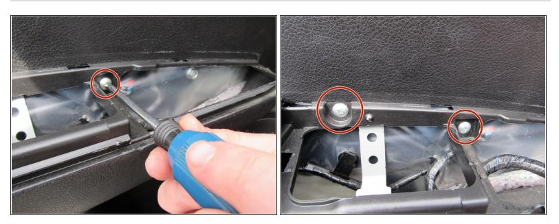
Unscrew both 8x3/4" Phillips screws from the middle of the door panel using your Phillips screwdriver.
