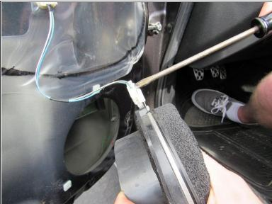
There will be a plastic adapter connecting wires to the speaker. To separate the adapter from the speaker, use a flathead screwdriver or spudger to pry the adapter off.
