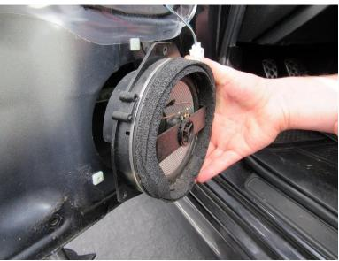
• There will be three 8x3/4" Phillips screws (the third screw is indicated by the arrow; you can't see the screw in the picture) keeping the speaker in place. Use a #0 Phillips screwdriver to remove them.
