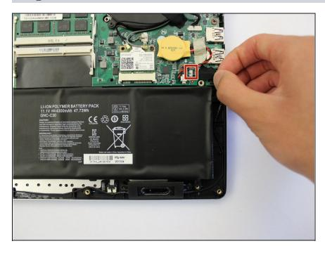
Unplug the connector by pulling on the wires.
