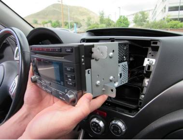
Remove the four 8x3/4" Phillips screws highlighted. Then slowly slide the stereo out from its housing.
