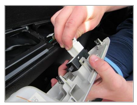
Remove the bundle of wires from the panel by pressing the tabs on the sides of the large white plastic connector.
