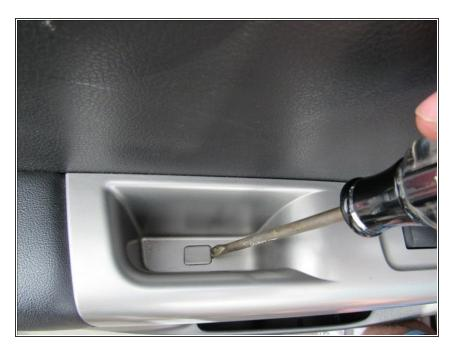
Use a flathead screwdriver to pry up the plastic tab inside the rear door armrest.
