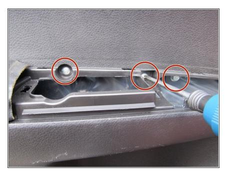
Use the Phillips screwdriver to unscrew the 8x3/4" screws behind the door handle panel that was just removed.
