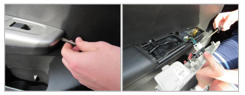
Use the flathead screwdriver to pry off and remove the panel over the door handle.
