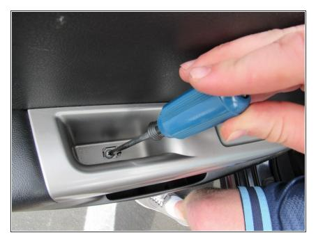
Use the Phillips screwdriver to unscrew the 8x3/4" Phillips screw inside the armrest.
