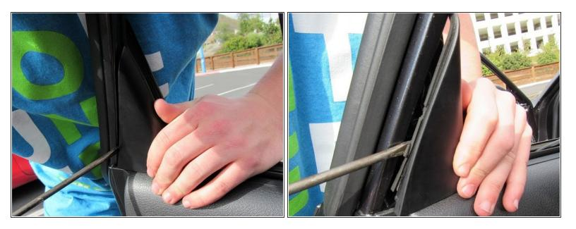
Use flathead to pry off the upper panel located at the top of the rear door panel.
