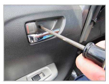
Pry off the plastic tab inside the rear door handle.
