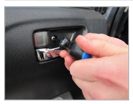
Use the Phillips screwdriver to unscrew the 8x3/4" Phillips screw inside the door handle.
