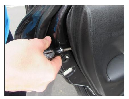
Use the flathead screwdriver to pry off the door panel, starting from the outside edge of the door.
