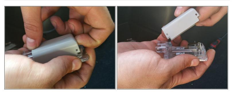
Remove back plate and switch from the unit to reveal the LED bulb.
