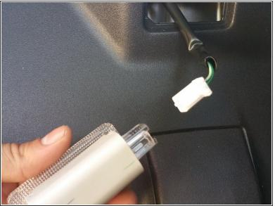
Remove the lighting unit from the plastic header by pressing inward on the side tabs and pulling outward.
