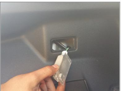
Remove clear plastic housing using a pry tool.
