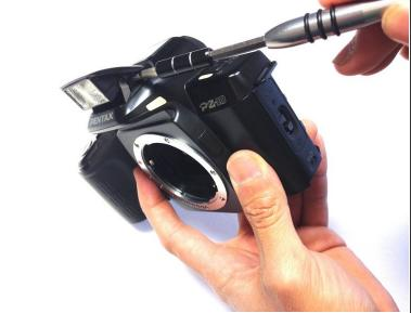
• Remove the two 5.5 mm JIS #0 screws on the sides of the flash assembly.
