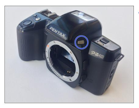
With the camera facing you, open the flash bulb by pushing the grey button to the right of the logo.
