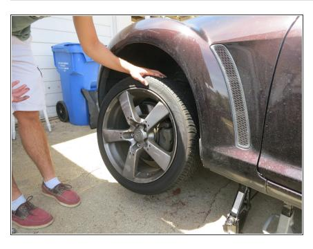
Remove all lug nuts holding the wheel on the car.
