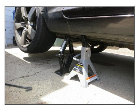
Put the jack stand under the car to ensure the car will not fall back down while you are working on it.
