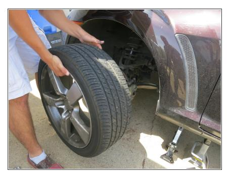
Remove the front wheel from the vehicle.
