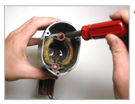
Remove the two 1" flathead screws located at the top and bottom of the motor housing.
