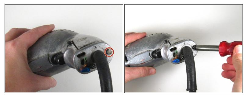
● Use the socket wrench to remove the 0.5" length screw from the bottom of the handle.
