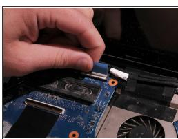
Disconnect three cables by pulling upward on black or blue tabs connected to them.
