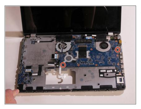
Remove the two 4.5mm Phillips screws from the system board
