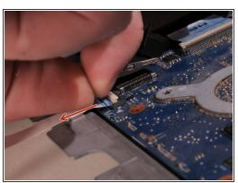
Disconnect cable by using a Flathead screwdriver to gently pry it off the black connector towards you.
