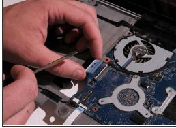
Disconnect three cables by lifting a white clamp with a Flathead screwdriver and pulling on the blue tab.
