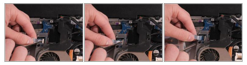
• Carefully disconnect the connecting cable by lifting the white clamp with a Flathead screwdriver and pulling on the blue tab away from connector.
