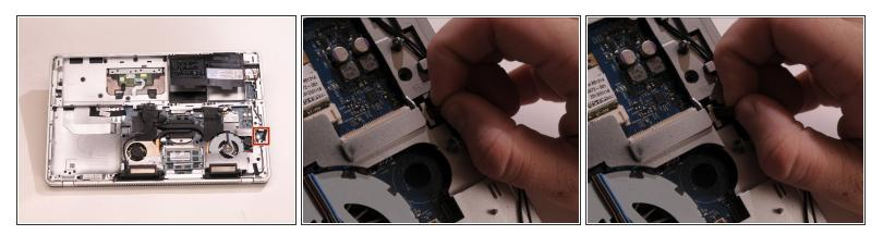
Remove the second connector by gently pulling upward.
