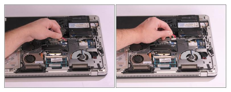
• Disconnect the multi-colored battery cable from the main assembly by gently pulling upward on it.
