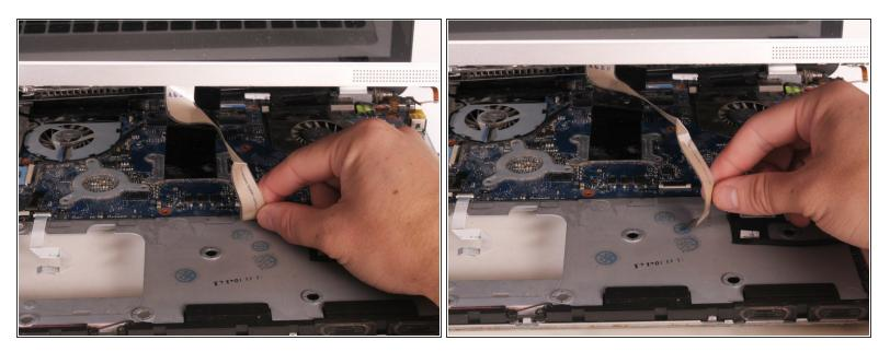
Gently pull the white connector shown in the picture towards you to disconnect it from the system board.
