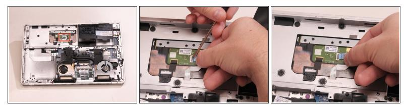
Remove the first connector by lifting the white clamp with a Flathead screwdriver and pulling the connector to your right.
