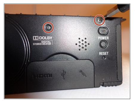
Remove the two 5mm screws from the panel to the right of the LCD screen.
