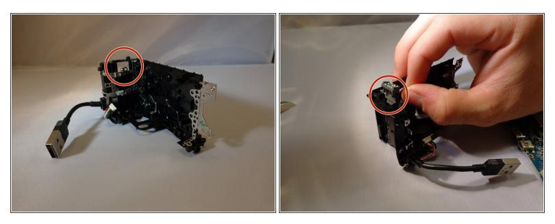
• Unplug the battery port connected to the frame/motherboard. Remove the battery port.
