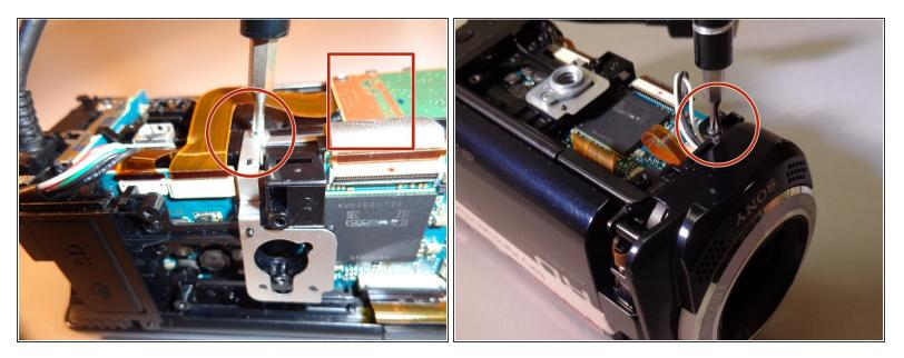
Remove the three black 5mm screws and one silver 4mm screw located on the front right-side of the camera, near the orange motherboard.
