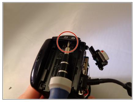
Use a Phillips #00 screwdriver to remove the one 3mm and two 5mm screws located in the battery assembly area.
