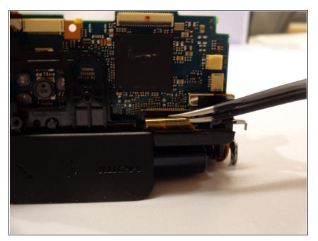
Slightly angle the mother board and remove the LCD screen by unplugging the remaining orange wire from the mother board.
