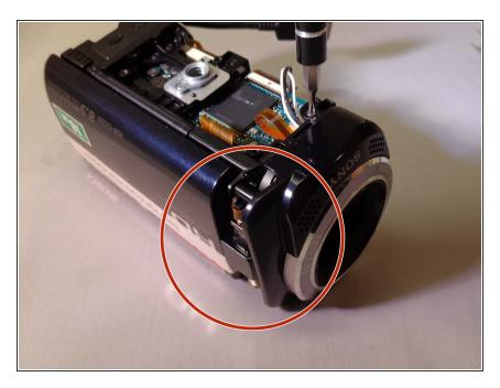
• Use a spudger to remove the LCD joint cover.
