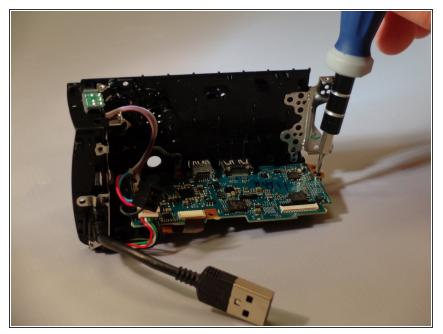
• Using a screwdriver unscrew 1 black 5mm screw from the mother board.
