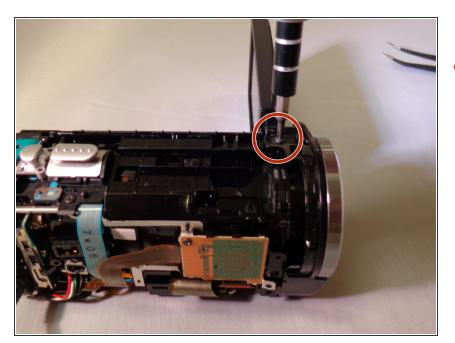
Remove the 5mm screw located on the top left near the camera lens.
