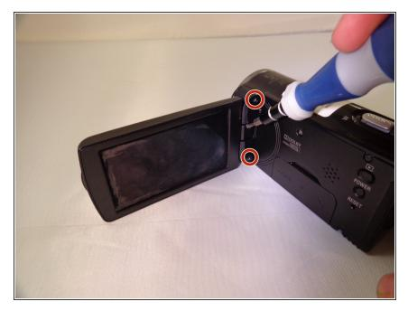
Unscrew near the front LCD joint of the camera 2 black 5mm screws and 1 black 3mm screw.
