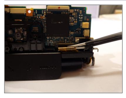
Slightly angle the mother board and remove the LCD screen by unplugging the remaining orange wire from the mother board. Removes the LCD screen and wire assembly connected to the mother board.
