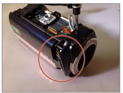
Use a spudger to remove the LCD joint cover.
