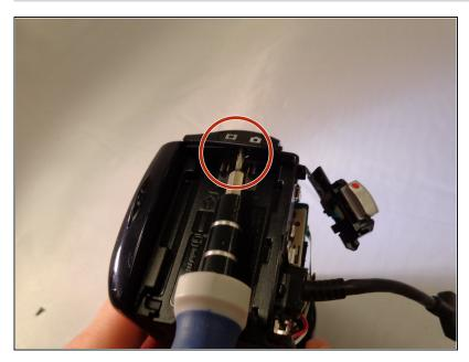
Use a Phillips #00 screwdriver to remove the one 3mm and two 5mm screws located in the battery assembly area.
