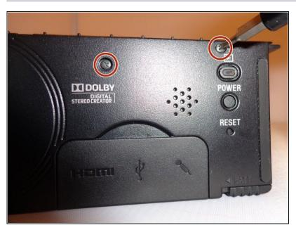
• Remove the two 5mm screws from the panel to the right of the LCD screen.
