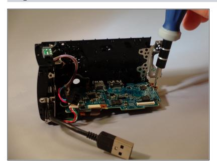
Using a screwdriver unscrew 1 black 5mm screw from the mother board.
