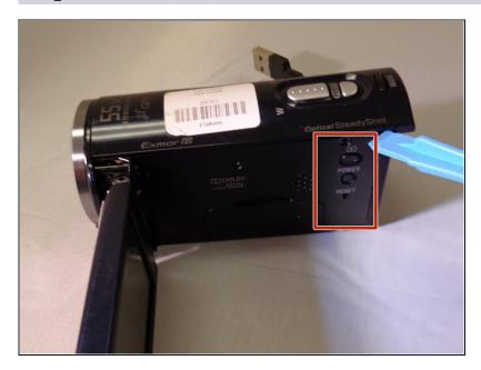
Use the plastic opening tool to remove the cover for the recording buttons.
