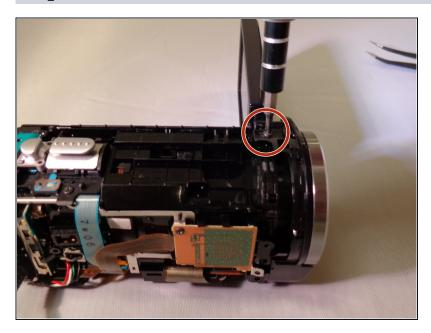
Remove the 5mm screw located on the top left near the camera lens.
