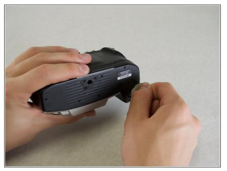
Use the edge of a coin to twist open the battery compartment on the bottom of the camera. (Twist counterclockwise)
